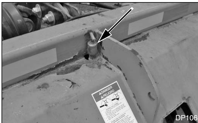
Figure 22. Gearbox Oil Fill Location
